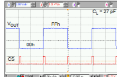
FIGURE 2-16: Full-Scale Settling Time.
