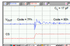
FIGURE 2-15: One Position Settling Time.
