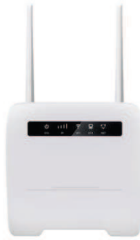
Figura N°50: CPE iStartek indoor cat4 LTE WiFi.
