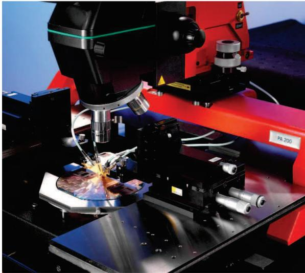
Figura 2.14: Foto de la Probe Station SÜSS MicroTec PM8®.
