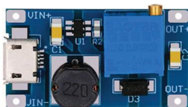
Figura 80 - Conversor DC/DC *Boost* MT3608.
