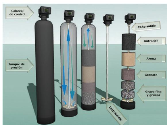
Figura 2-5: Diagrama filtro multimedia. Adaptado de: <http://neyawatersolutions.com/press.php>
