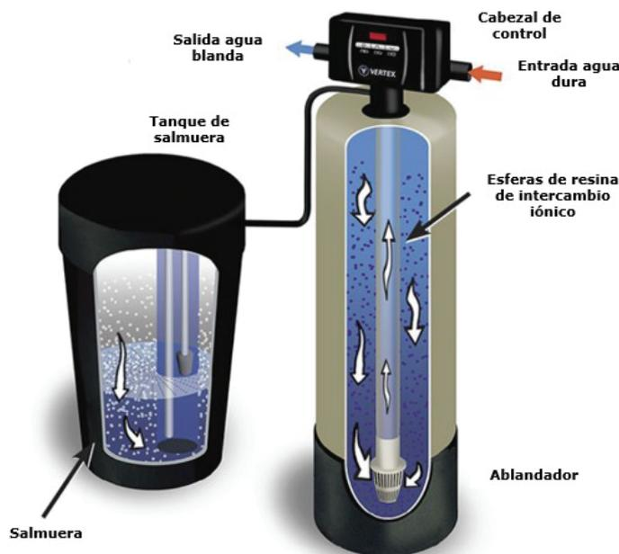
Figura 2-6: Esquema ablandador. Adaptado de: <https://vertexwater.com/how-a-water-softener-works/>
