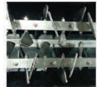
304 stainless steel paddle construction.
